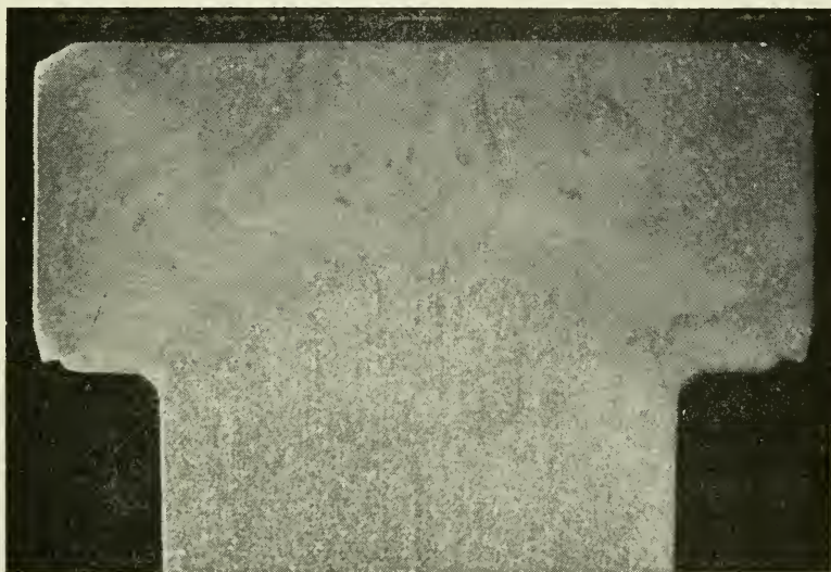
Fig. 17-3. Fiber structure in wrought product revealed by macroetching. 5 \times .
