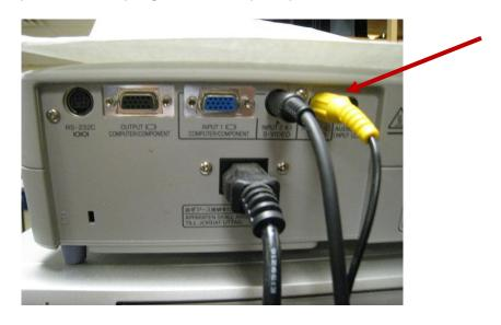
NOTE: You will be using an A/V cable with red, white, and yellow plugs at each end. The yellow is for video input, and the red and white plugs are for sound.
