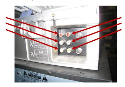
Step 5: Plug the other end of the cable (red, white, and yellow pieces) into the back of the VCR/DVD Player at the corresponding ports.
