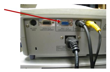
Step 2: Plug the computer cable into the projector, tightening the screws to secure it in place.
